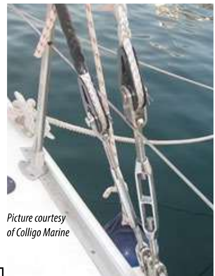
Figure 4: HPME stranded rope rigging (Dynice DUX) spliced around special thimbles and attached to (turnbuckles) rigging screws. It should be noted that the shroud in the foreground (without black chafe protection can easily be fully inspected.
